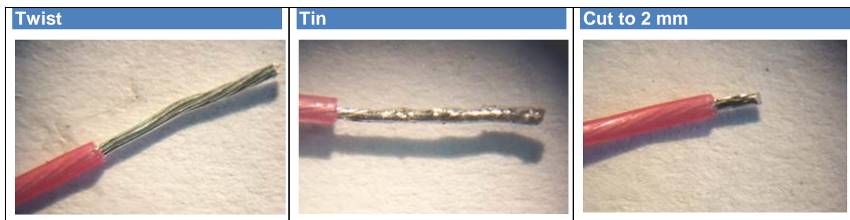
Figure 4: Wire preparation steps (schematic)
